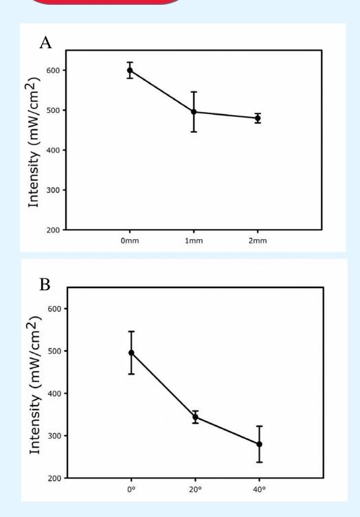
**Figure 1:** relationship between light intensity and A distance from sensor or B: light intensity and angle to the sensor
